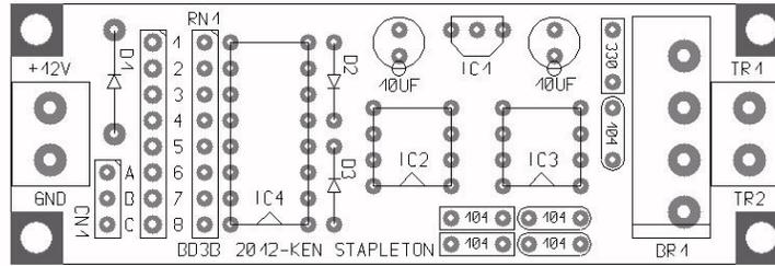
*FIGURE 1 - CIRCUIT BOARD LAYOUT*
