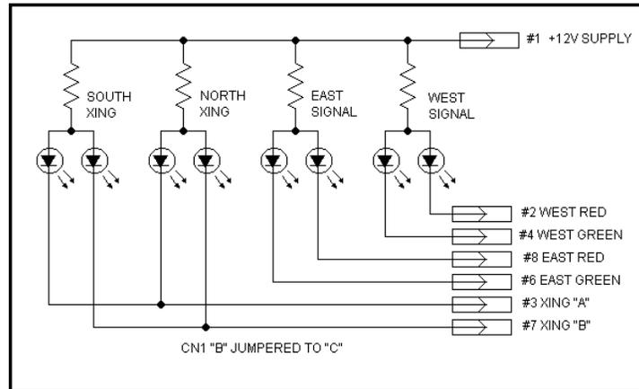
*FIGURE 5 - CN1 "B" JUMPERED TO "C"*
